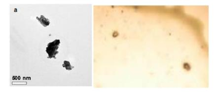
From the measurement results with the size anlizer particle (PSA) it was found that with the change of time it was found that the average particle size decreased, partly increased the size when viewed in Figure 4 because it collected some particles into one so it was detected bigger. So that measured is the rearata. Size becomes important if it sees an influence in nanomedicine in its application as a photodynamic sensitizer (Alyssa et al, 2013).
